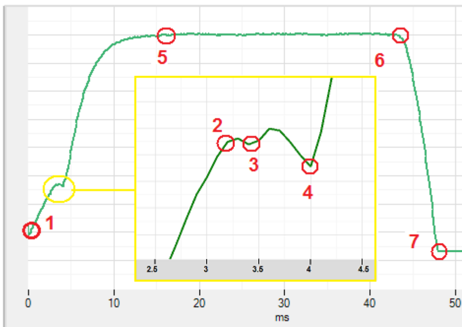
Figure 1. Opening (trip) coil current waveform with the zoomed part
